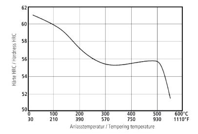
Hardening temperature:  $1030^{\circ}\text{C}$  /  $1886^{\circ}\text{F}$  Specimen size: square 20 mm
