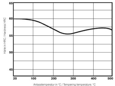
Hardening temperature:  $1030^{\circ}\text{C}$  /  $1886^{\circ}\text{F}$  Specimen size: square 20 mm
