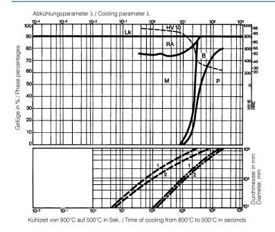
HV10... Vickers Hardness Lk... Ledeburite carbide RA... Residual austenite M... Martensite B... Bainite
