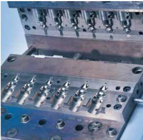
The development of ever-larger plastic parts increases complexity of heat treatments of the moulds. In order to eliminate dimensional changes and quench cracking, prehardened steels are used for large tools. They are heat-treated to a hardness of 290 – 400 HB / approx. 30 – 40 HRC by BÖHLER. At this hardness, steel retains its good machinability but still has good wear resistance and adequate strength.
